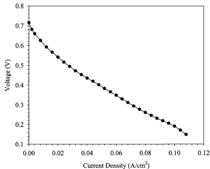
**Figure 6.** DME polarization curve with Nafion 115 electrolyte. Test conditions: cell temperature: 90°C, fully humidified DME anode and cathode, anode/cathode pressure: 1/1 atm,  $\xi_{\text{DME}}$ : 0.5 A/cm<sup>2</sup> equivalent (constant flow rate),  $\xi_c$ : 0.35 A/cm<sup>2</sup> equivalent (constant flow rate).
