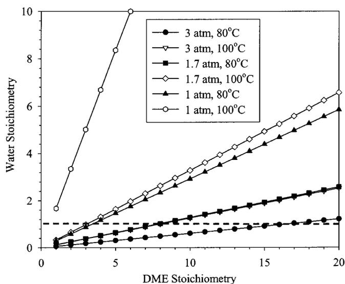
**Figure 2.** Plot of DME fuel cell inlet stoichiometry vs. fuel cell inlet water stoichiometry as a function of operating pressure and temperature, assuming fully humidified anode inlet flow. A dashed line is shown for water stoichiometry of unity.
