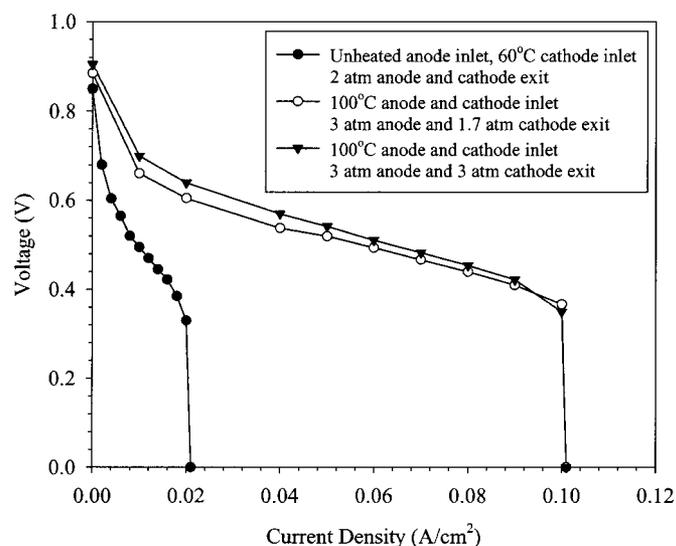
**Figure 4.** Polarization curves as a function of temperature and cathode pressure. Nafion 117 electrolyte. Common conditions: unhumidified cathode,  $\xi_{\text{DME}}$ : 1.875 A/cm<sup>2</sup> equivalent (constant flow rate),  $\xi_c$ : 1.875 A/cm<sup>2</sup> equivalent (constant flow rate).
