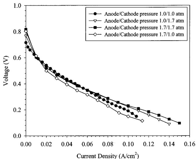
**Figure 7.** DME polarization curve with Nafion 115 electrolyte for various anode and cathode pressures. Test conditions: cell temperature: 90°C, fully humidified DME anode and cathode,  $\xi_{\text{DME}}$ : 0.5 A/cm<sup>2</sup> equivalent (constant flow rate),  $\xi_c$ : 0.35 A/cm<sup>2</sup> equivalent (constant flow rate).
