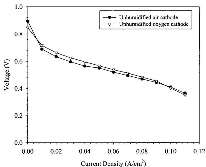
**Figure 5.** DME polarization curves as a function of cathode oxygen mole fraction. Nafion 117 electrolyte. Test conditions: cell temperature: 100°C, fully humidified DME anode, unhumidified air cathode, anode/cathode pressure: 3/1.7 atm,  $\xi_{\text{DME}}$ : 1.875 A/cm<sup>2</sup> equivalent (constant flow rate),  $\xi_c$ : 1.875 A/cm<sup>2</sup> equivalent (constant flow rate).
