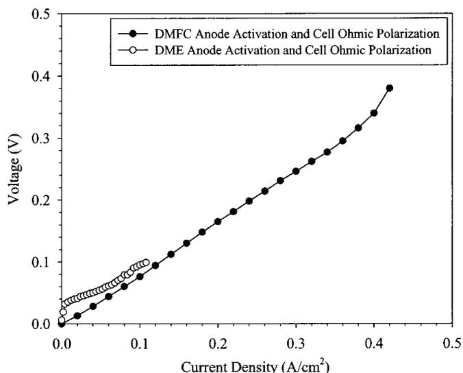
**Figure 10.** Activation plus ohmic polarization comparison between DMEFC and DMFC with Nafion 115 electrolyte. Test conditions: cell temperature: 90°C, fully humidified DME anode and cathode, anode/cathode pressure: 1.0/1.0 atm,  $\xi_{\text{DME}}$ : 0.5 A/cm<sup>2</sup> equivalent (constant flow rate),  $\xi_c$ : 0.35 A/cm<sup>2</sup> equivalent (constant flow rate).
