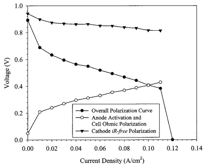
**Figure 8.** DME individual and overall electrode polarization curves with Nafion 117 electrolyte. Test conditions: cell temperature: 95°C, fully humidified DME anode and cathode, anode/cathode pressure: 3/1.7 atm,  $\xi_{\text{DME}}$ : 0.5 A/cm<sup>2</sup> equivalent (constant flow rate),  $\xi_c$ : 0.35 A/cm<sup>2</sup> equivalent (constant flow rate).
