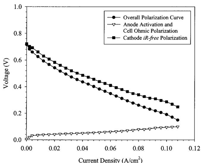
**Figure 9.** DME individual and overall electrode polarization curves with Nafion 115 electrolyte. Test conditions: cell temperature: 90°C, fully humidified DME anode and cathode, anode/cathode pressure: 1.0/1.0 atm,  $\xi_{\text{DME}}$ : 0.5 A/cm<sup>2</sup> equivalent (constant flow rate),  $\xi_c$ : 0.35 A/cm<sup>2</sup> equivalent (constant flow rate).
