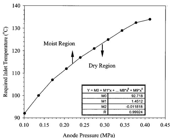
**Figure 3.** Relationship between anode pressure and fully humidified anode inlet temperature to satisfy required 3:1 molar ratio for electrochemical reaction. This assumes no net drag of water from anode to cathode and all water is supplied to the anode by fully humidified vapor-phase water. Above the curve, there is adequate water for reaction, below the curve, there will not be adequate water for electrochemical oxidation of DME.
