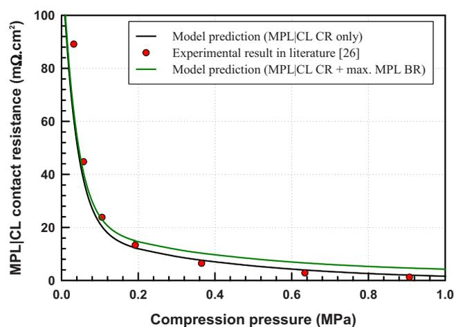
**Figure 4.** (Color online) Predicted MPL|CL CR vs applied CP. Model results for SGL 10BB (MPL|CL CR only and MPL|CL CR + maximum MPL BR) and experimental results for TGP-H-060 (with applied MPL) given in Ref. 26 are compared. The MPL on both materials have similar material properties and roughness values.<sup>42,c</sup> The DM material properties used are identical and equal to that of TGP-H-060.<sup>49</sup>
