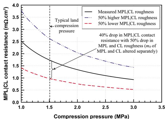
**Figure 6.** (Color online) Predicted MPL|CL CR vs CP for different degrees of MPL and CL roughness.
