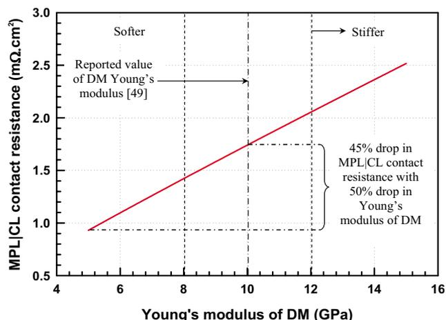
**Figure 7.** (Color online) Effect of the Young's modulus of the backing DM layer on the predicted MPL|CL CR for homogeneous CP of 1.5 MPa (under a typical land).
