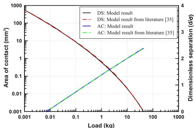
**Figure 3.** (Color online) Verification plot of area of contact (AC) and dimensionless separation (DS) vs the applied load (comparing current model results with the data reported in the literature<sup>35</sup>).
