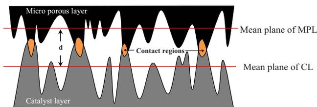
**Figure 1.** (Color online) Two-dimensional schematic of the MPL/CL interfacial contact.
