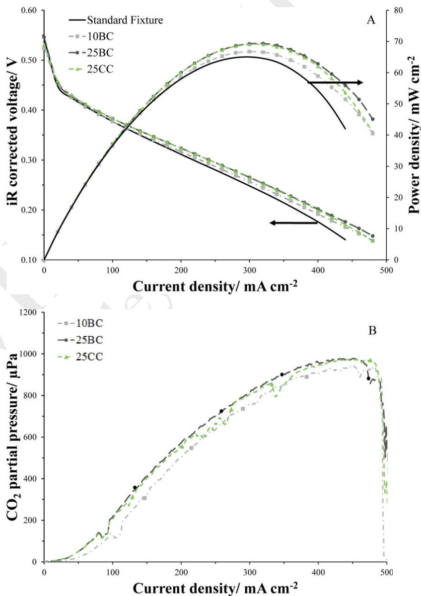
Fig. 2 DFAFC polarization curves comparing the standard solid plate flow field to the advanced anode selectively gas permeable flow field (SGPF) at 40 °C with 5 M formic acid (2.5 mL min<sup>-1</sup>) on the anode and air (21% O<sub>2</sub>, 0.5 L min<sup>-1</sup>) as the cathode feed. The separators in the anode SGPF were SGL 10BC, 25BC, and 25CC. (A) Polarization and power density and (B) CO<sub>2</sub> partial pressure.
