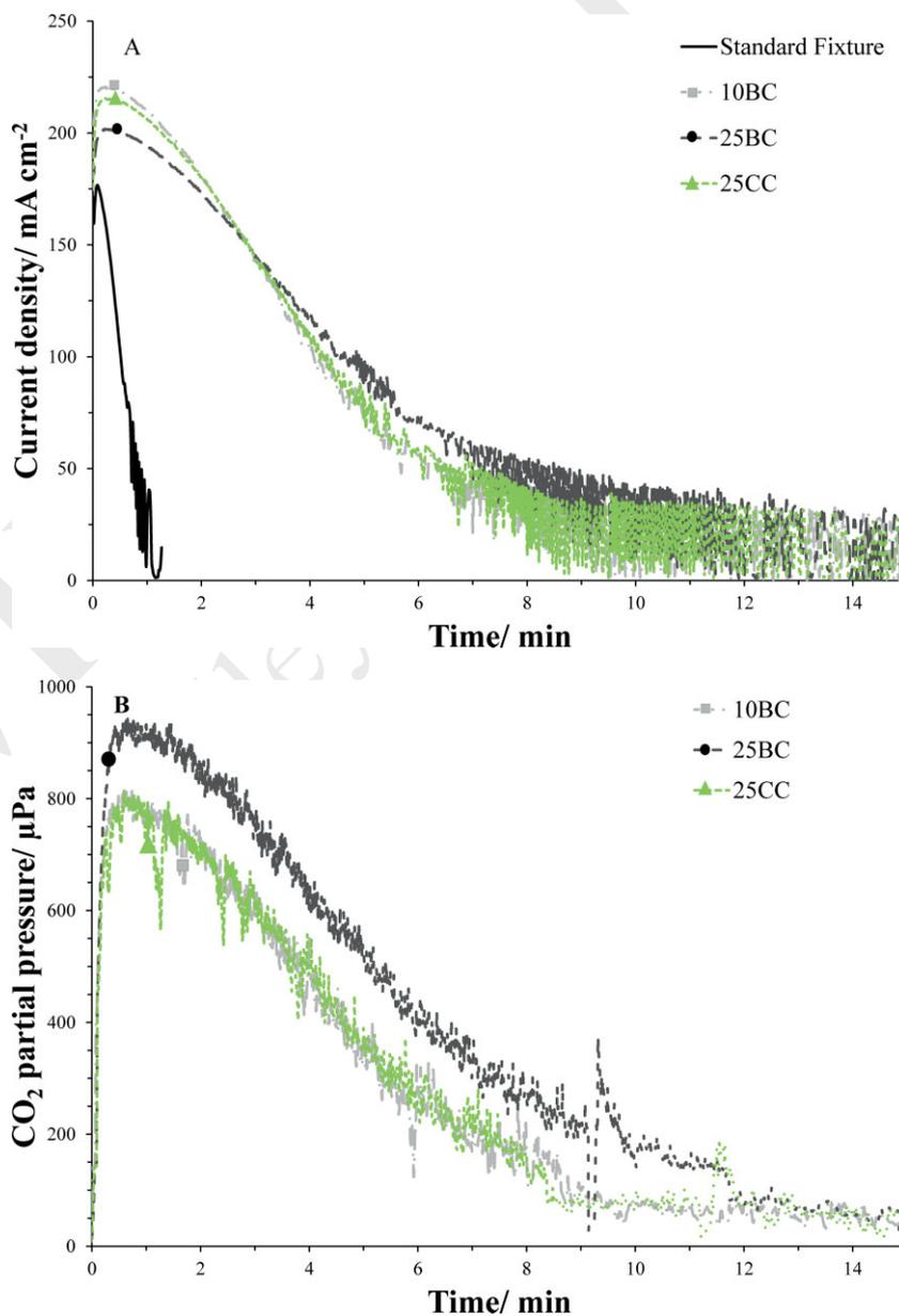
Fig. 3 Potentiostatic hold at 0.3 V comparing the standard solid plate flow field to the anode SGPF at 40 °C with 5 M formic acid (2.5 mL min<sup>-1</sup>) on the anode and air (21% O<sub>2</sub>, 0.5 L min<sup>-1</sup>) as the cathode feed. The separators in the anode SGPF were SGL 10BC, 25BC, and 25CC. (A) Current density and (B) CO<sub>2</sub> partial pressure.
