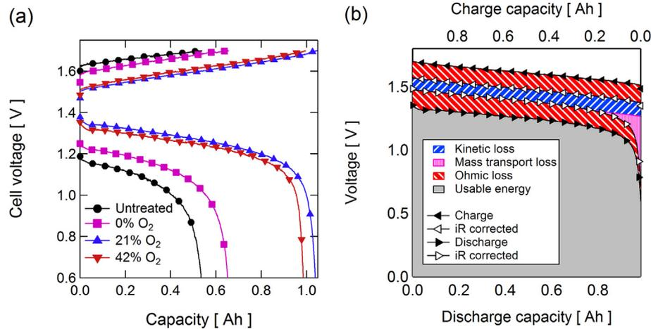
**Fig. 2.** Charge/discharge profiles obtained at  $200 \text{ mA cm}^{-2}$  for (a) untreated and 15 h treated samples and (b) 15 h enriched oxygen treated electrode with breakdown of losses from kinetic, ohmic, and mass transport polarizations.
