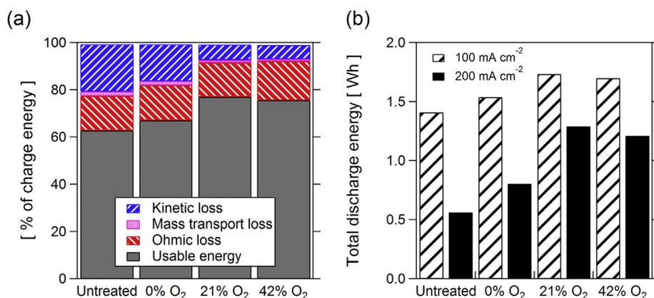
**Fig. 3.** Summary of cycling for untreated and 15 h treated samples: (a) usable energy and kinetic and ohmic losses at  $200 \text{ mA cm}^{-2}$  and (b) total discharged energy at  $100 \text{ mA cm}^{-2}$  and  $200 \text{ mA cm}^{-2}$ .
