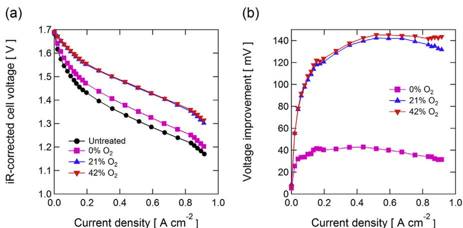
**Fig. 1.** (a) *iR*-corrected polarization curves for untreated carbon paper and those treated for 15 h in 0%, 21%, and 42% oxygen environments and (b) *iR*-corrected voltage improvement of each heat treatment relative to untreated carbon paper.
