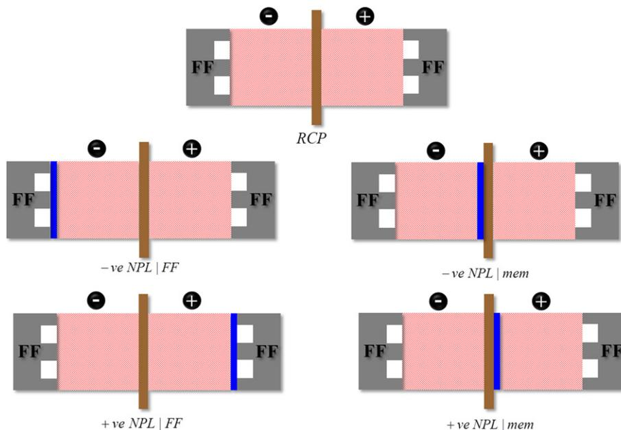
**Fig. 1.** A schematic of the nanoporous layer (NPL) orientations tested. The solid blue region represents the NPL, the hashed region represents carbon paper, the brown separator represents the membrane (mem), and the flow field (FF) is as labeled (not to scale). (For interpretation of the references to colour in this figure legend, the reader is referred to the web version of this article.)
